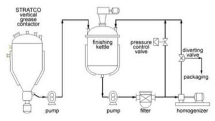
An alternate procedure is to partially or completely finish the grease in the Contactor reactor. This option takes advantage of the high shear milling action of the Contactor reactor's impeller. Lighter greases can be completely finished in the Contactor™ reactor and then directly packaged.
